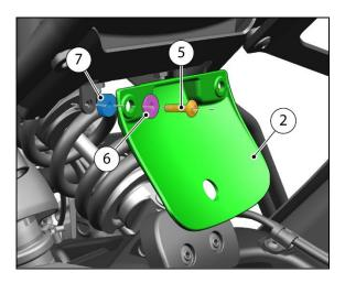
4. Tighten the screws M5x20 (5) to a torque of <u>5 Nm ± 10%</u>.
