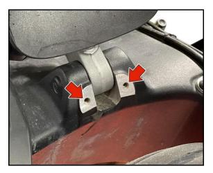
Clean the threads of the M5x9 screws previously removed from the rear mudguard and apply Loctite 243.
