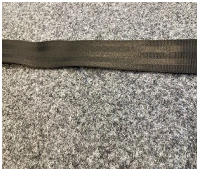
Figure 2. Waviness indicates that the seat belt was pulled on when exiting the rear of the vehicle
