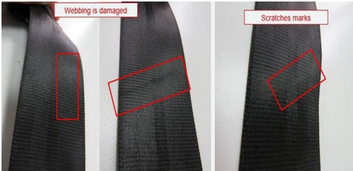
Figure 1. Marks indicating that the seat belt was trapped in the front door
