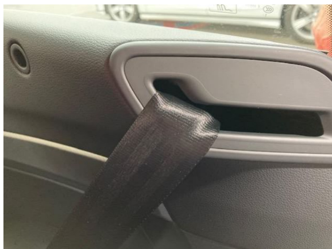
Figure 3. Pulling on the seat belt when exiting the vehicle can damage the seat belt/microphones.
