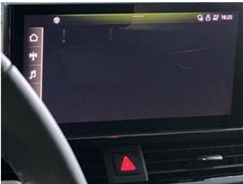
Figure 1: ASI display is blank when using wACP.
