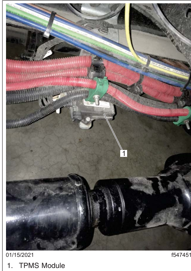
Fig. 1, Location of the TPMS Module
