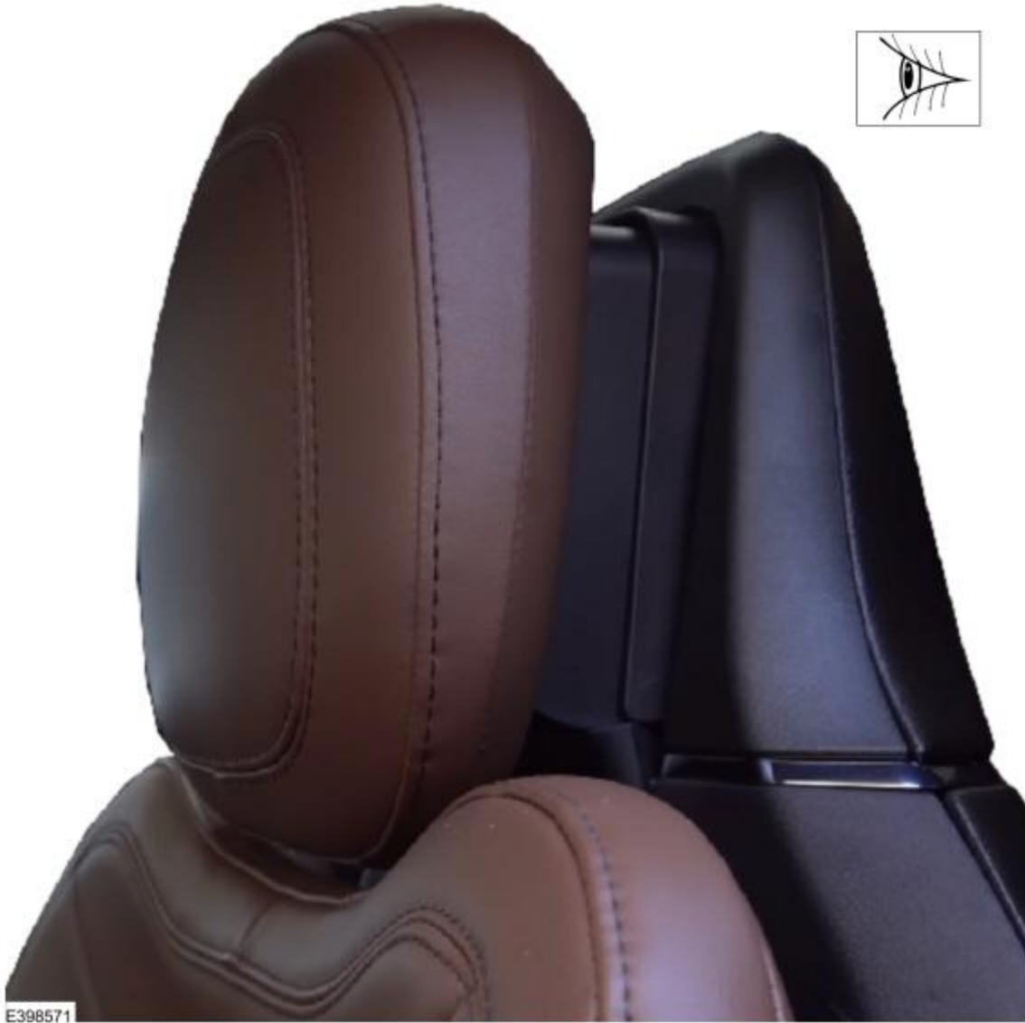
Figure 2 - Second generation head restraint
