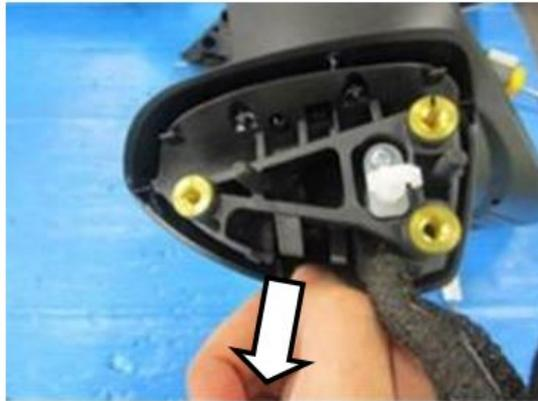
5. Peel off the two seal packing (1) from the harness.
