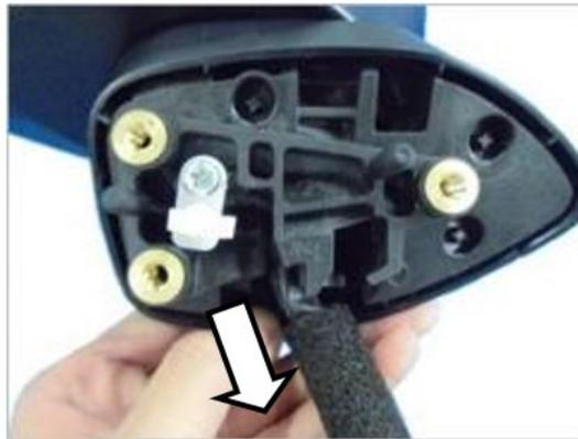
5. Peel off the two seal packing (1) from the harness.
