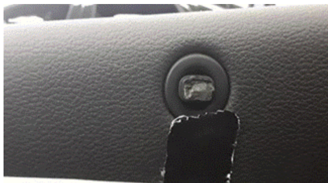
Figure 1. The wind deflector bearing pin is broken off in the mount.
