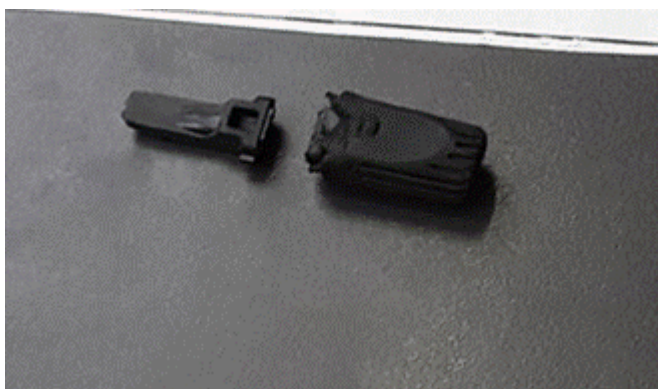
Figure 3. Removed pieces of the broken wind deflector bearing pin.
