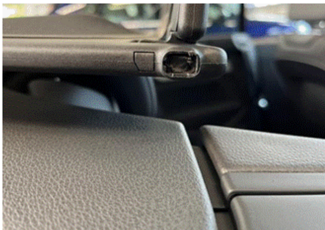
Figure 2. The wind deflector bearing pin is broken off of the deflector structure.
