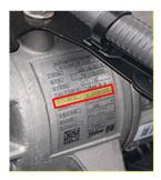
**IMPORTANT:** The NEW part CANNOT be identified by the Part Number. The production date code located on the compressor must be used. In this example (112835535), the "1" indicated the production year as 2021 (a "9" would be 2019, etc.). The next 2 digits, "12" indicate December as the production month ("01" would be January, etc.).
