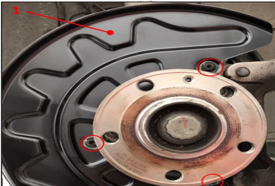
Figure 1. Splash plate for brake disc with contact surfaces of securing bolts.
