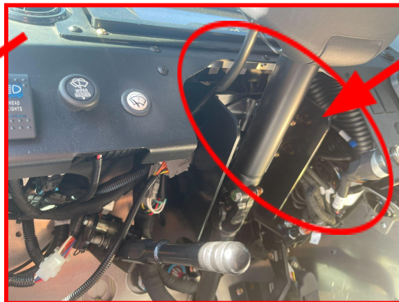
Image 3 - Harness can be located on this side of the steering column
