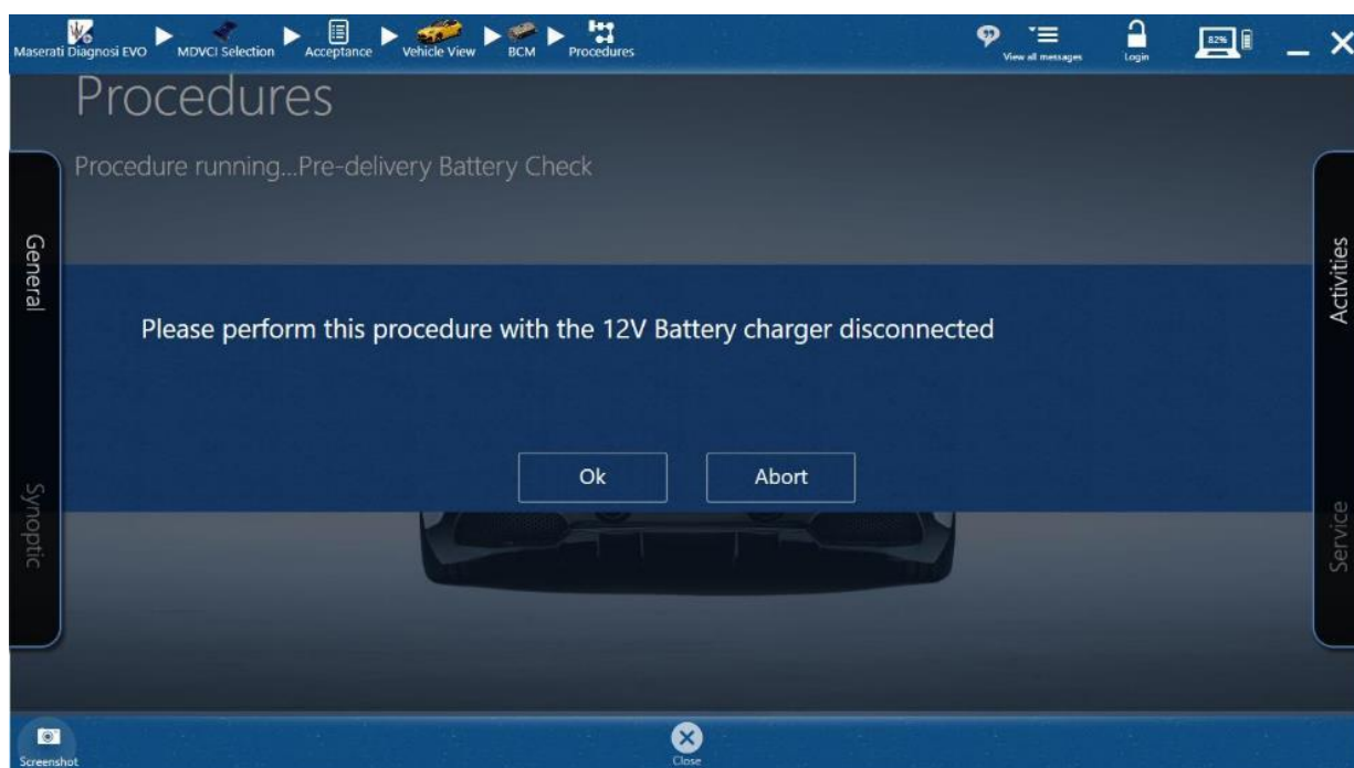
Figure 3: warning message in case a Battery charger or maintainer is connected.
