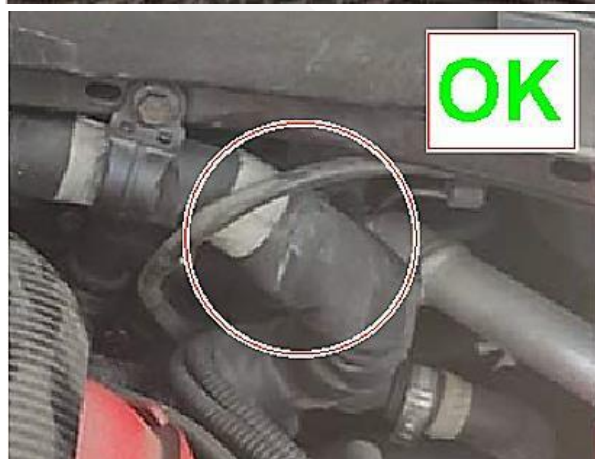
Example of correct routing IN FRONT of the plate
