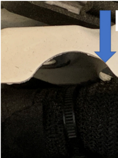
Close up of area where harness may chafe.
