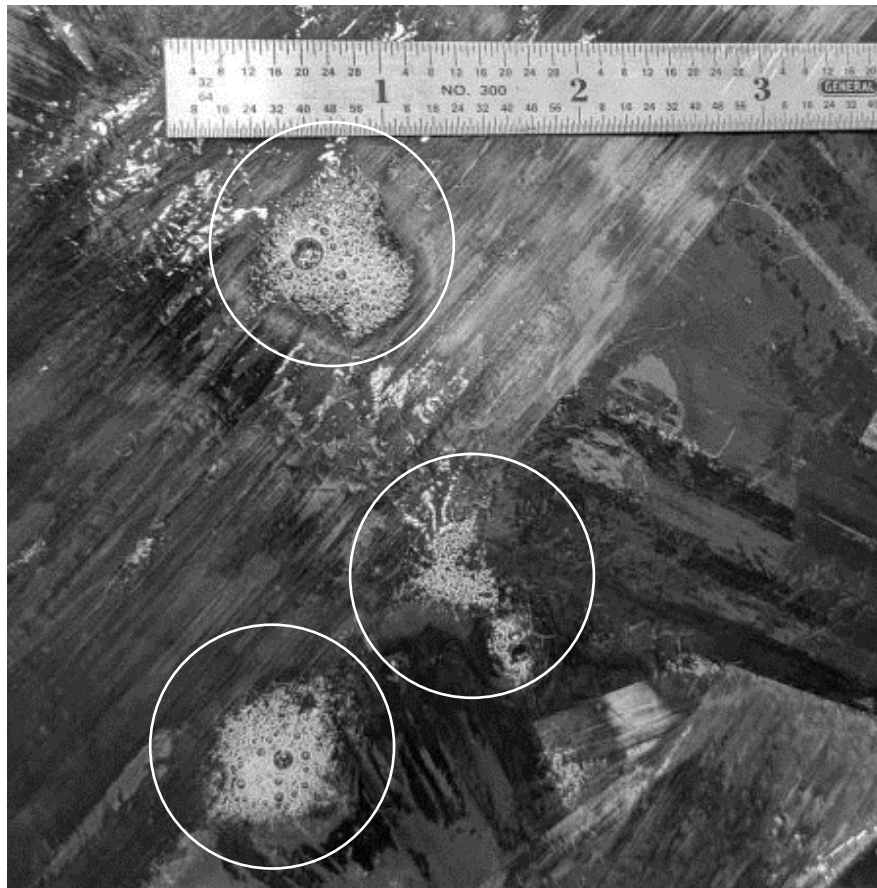
FIGURE 11. Solidified resin bubbles on the cylinder surface ( circled ).
