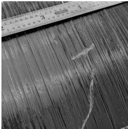
Figure 5. Gouge in the composite categorized as Level 2b abrasion damage.
