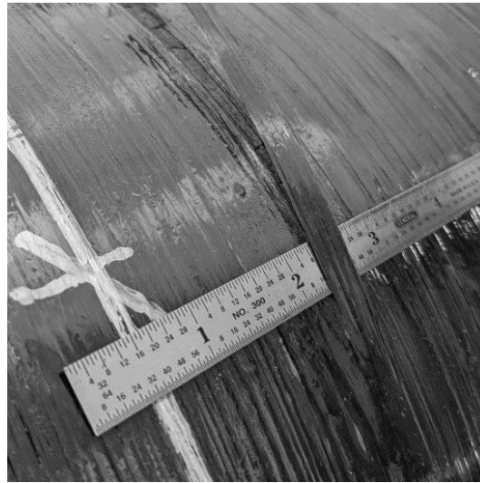
FIGURE 9. Fiber unraveling with a section of the composite lifted up
