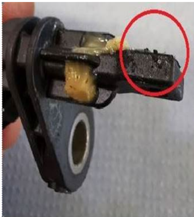
Figure 2: Metallic particles in the speed sensor.
