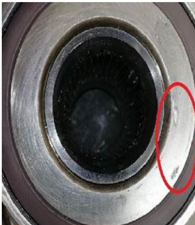
Figure 5: Metallic particles/damage in the wheel hub/bearing.
