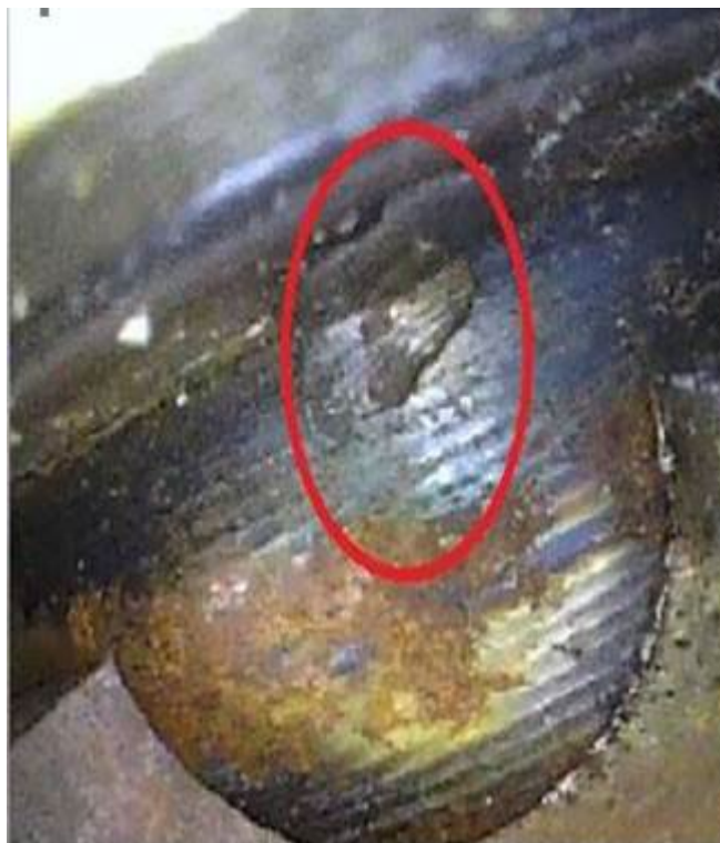
Figure 3: Metallic particles in the hub.
