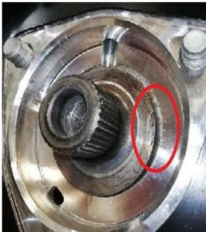
Figure 4: Metallic particles/damage in the wheel hub/bearing.
