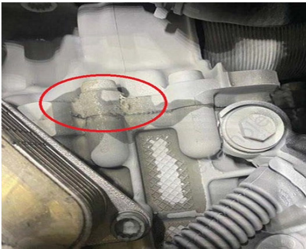
Figure 1. Oil leak at transmission case seam.
