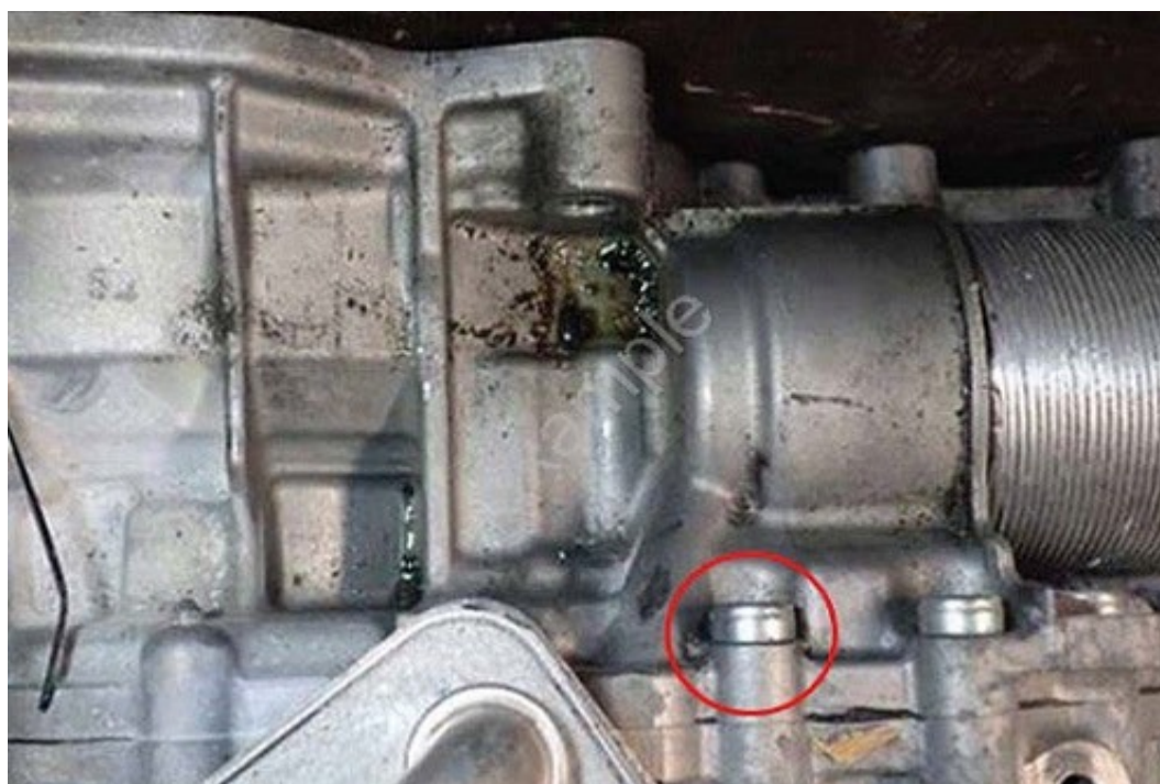
Figure 2. Housing bolt leak.
