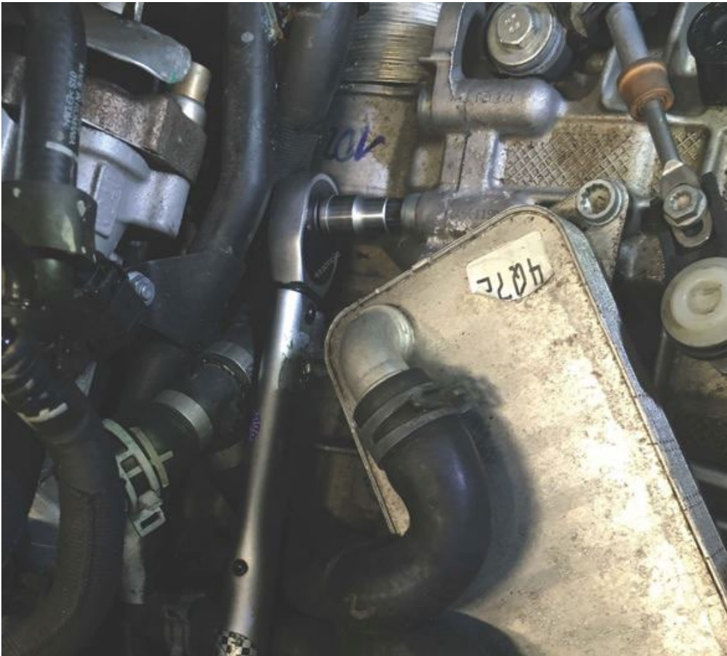
Figure 3. Tightening housing bolt to a torque of 20 Nm + 90° .
