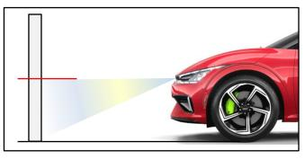
7. Check that each headlamp low beam aligns with the cutoff line previously marked.
