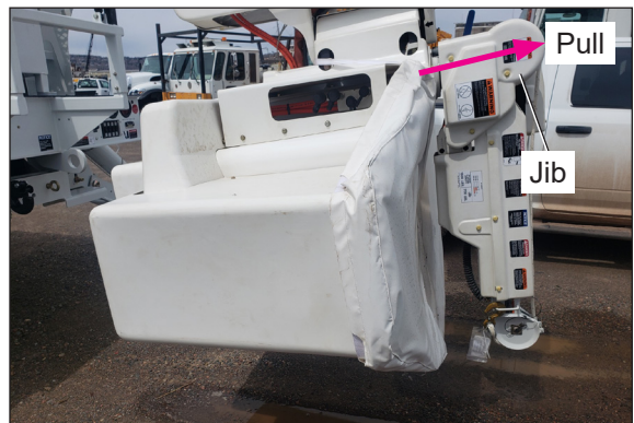
Figure 3 – Pulling on Jib
