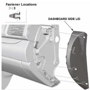
2. Remove the passenger's dashboard undercover, then disconnect the connector (for some models).
