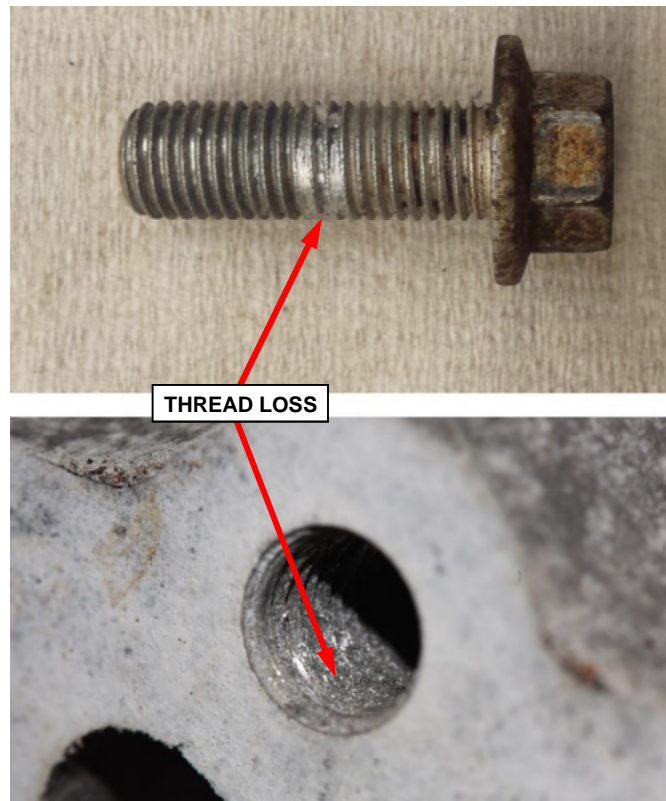
Figure 18 – Inspect for Thread Loss
