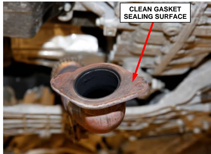
Figure 29 – Crossunder Pipe Flange
