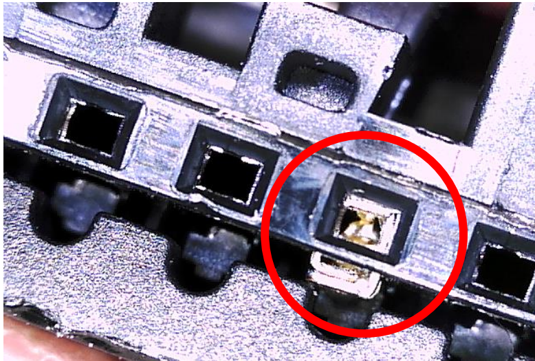
Misaligned Terminal In IP Harness D3944A
