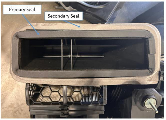
I.Inspect air inlet housing primary seal and verify the seal is properly installed (not rolled or deformed).
