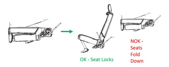
**Inspection:** Move the seat from the folded position to upright. Does the seat lock in the first locking position?
