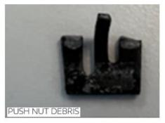
Example of a cracked and broken snap nut.
