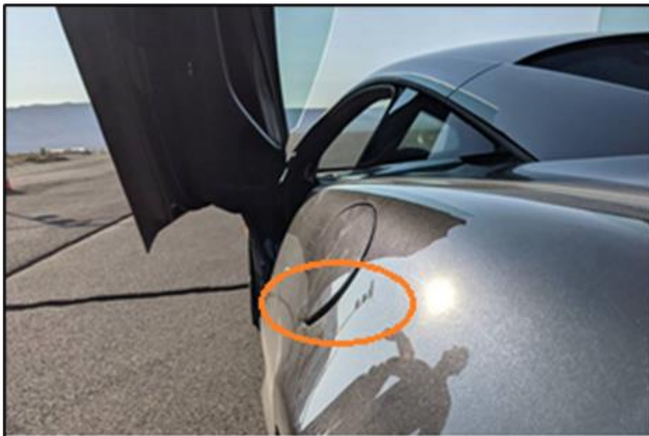
Image 1: PHEV Socket Cover (LH) – Rear Lower Edge Over Flush
