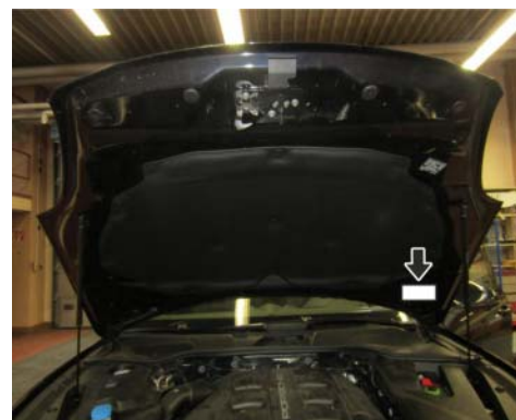
Proof of Completion Label: specified position (Exemplary illustration — Cayenne (9YA) position accordingly)
