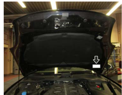
Proof of Completion Label: specified position (Exemplary illustration — Cayenne (9YA) position accordingly)
