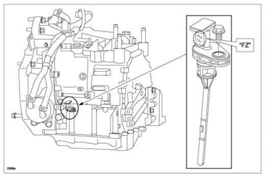
The fluid level should be between the (1) and (2) when the ATF is warm (at least 50 °C (122 °F)).
