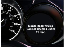
In the following cases, the MRCC with Stop & Go function system is canceled when the vehicle is traveling at 19 mph (30 km/h) or less:
