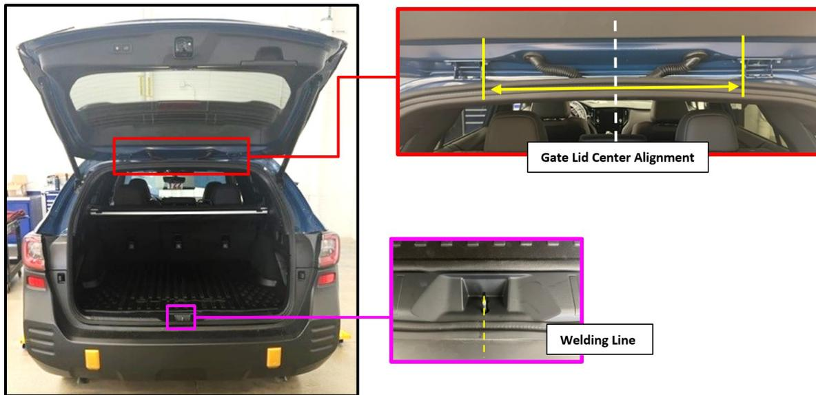
When installing the new seal, confirm the center of the gate lid and the welding line are aligned with one another as shown below.
