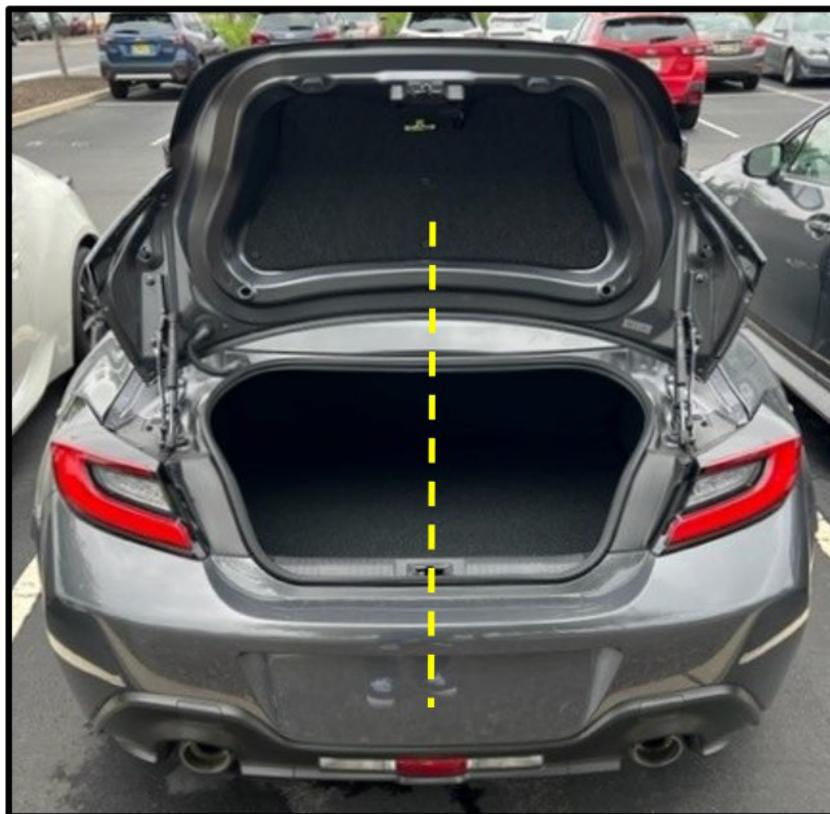
Confirm the entire weather strip is fully seated onto the body flange in all areas.
