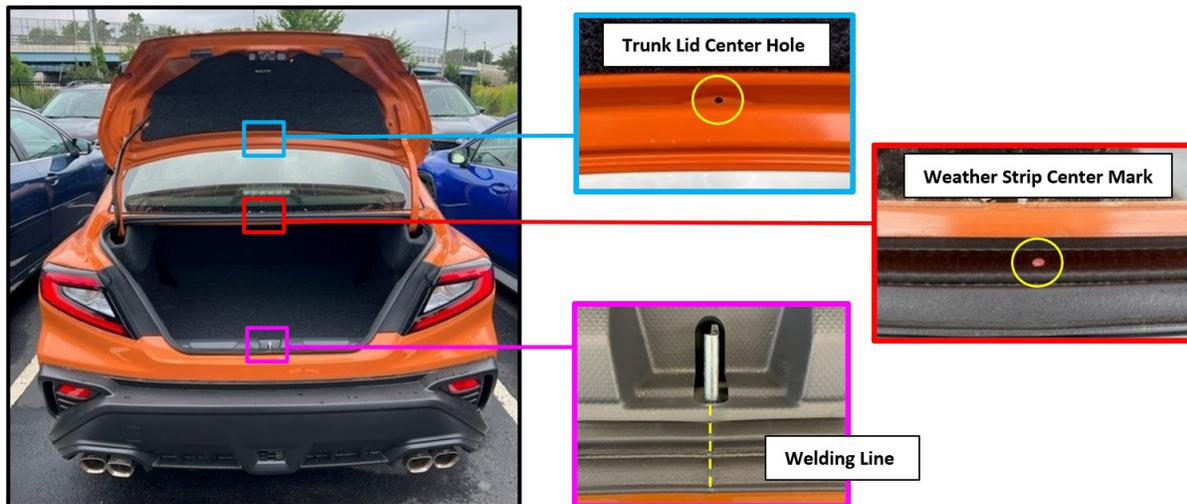
When installing the new seal, confirm the trunk lid center hole, the weather strip center mark and the welding line are all aligned with one another as shown below.
