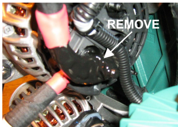
Figure 3: Black color guard on terminal post
