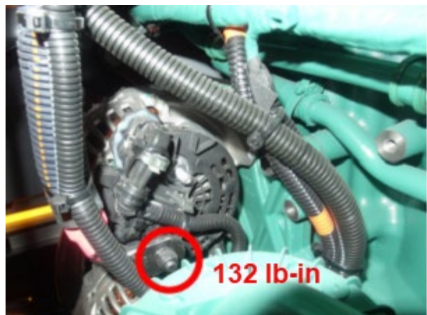
Figure 6: Torque top nut to 132 lb-in
