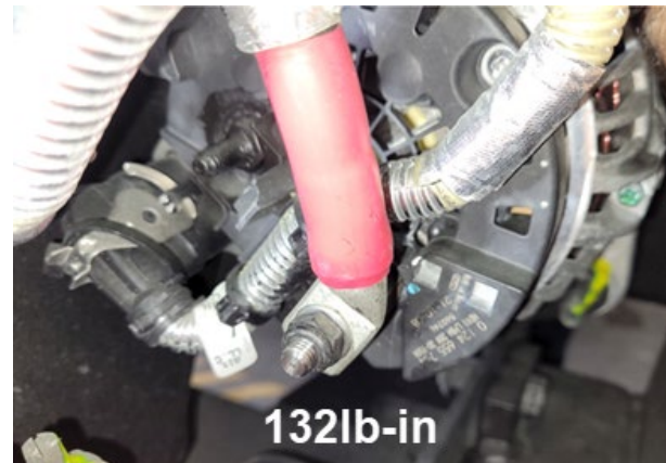
Figure 11: Torque top nut to 132 lb-in
