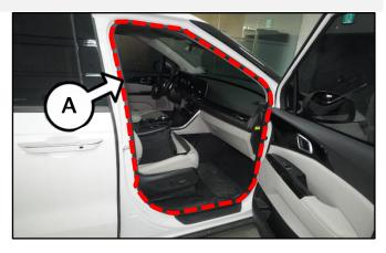
2. Install the new weatherstrip (A) securely into the channel around the door frame.
