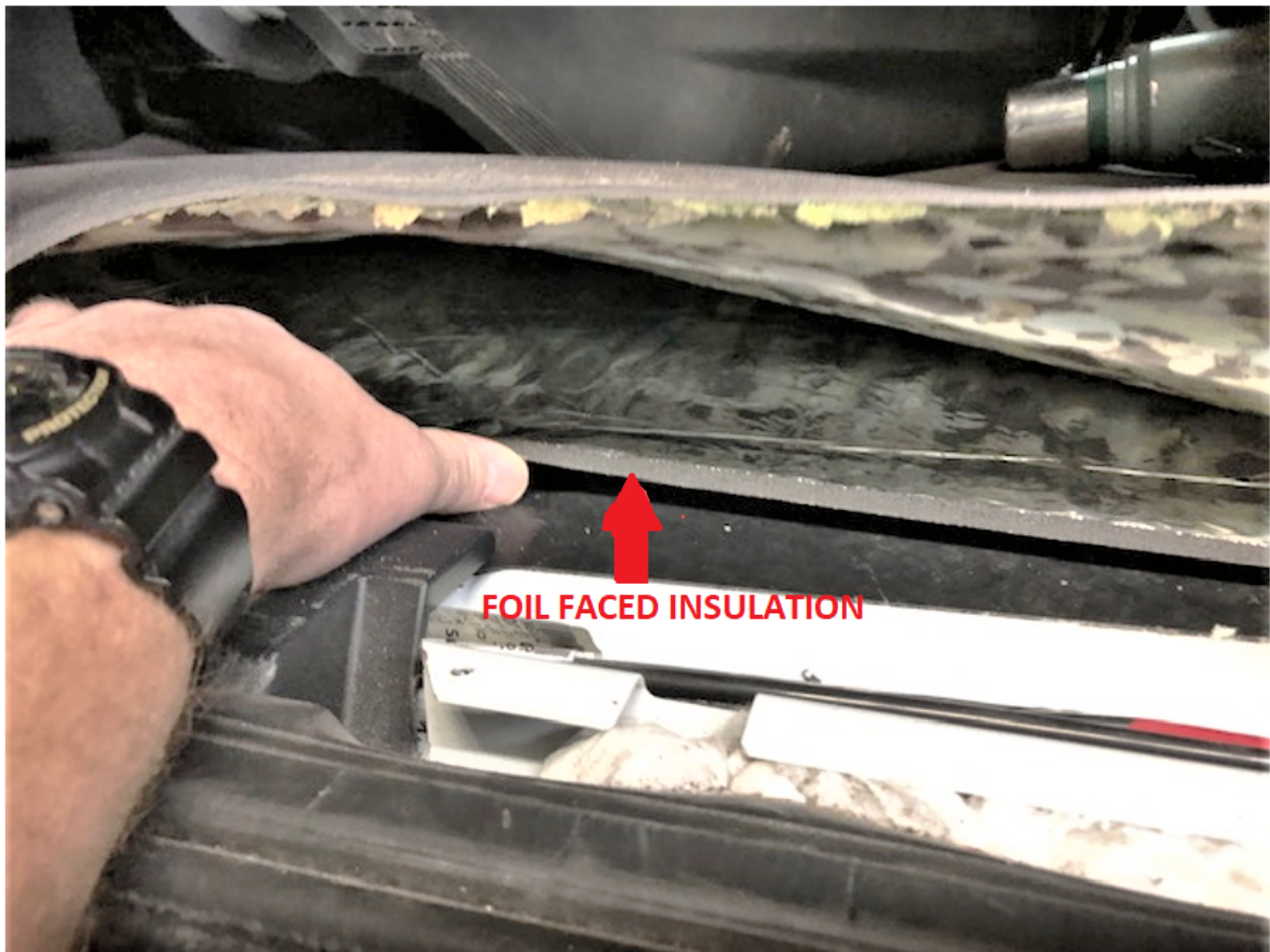
Figure 4 Added insulation (foil faced) to be removed as documented in figure 2 or figure 3 depending on the drive position.
