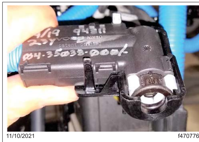
Fig. 3, Reinforcement Cap Installation
