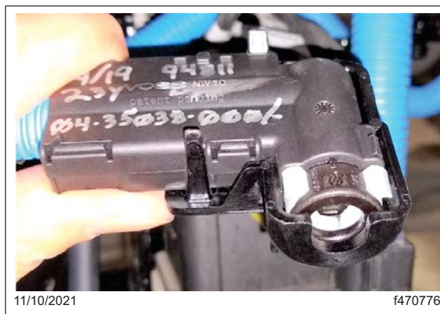
Fig. 3, Reinforcement Cap Installation
