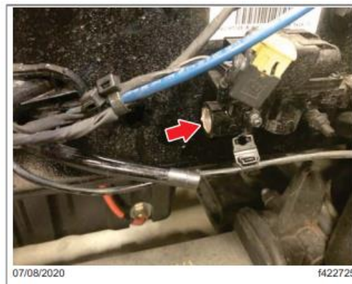
Fig. 6, Disconnecting the Quick Disconnect Fitting
