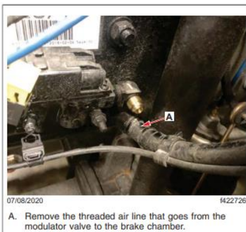
Fig. 7, Removing the Threaded Air Line
