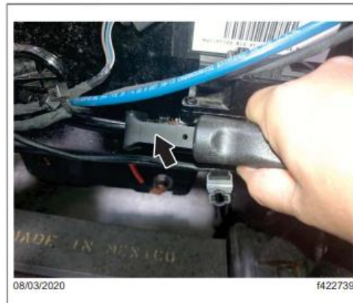
Fig. 5, Disconnecting the Plastic Air Line
