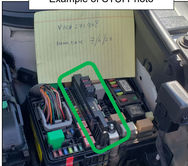
Correct multi-fuse. Fuse is taller, with protruding individual, replaceable fuses.
