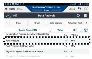
5. Shut off the engine and monitor the fuel pressure. If the pressure does not drop, this bulletin does not apply and continue with normal diagnostic for misfires.
