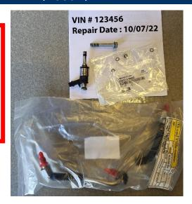
Install new combustion seals on all the reused injectors during reinstallation.
