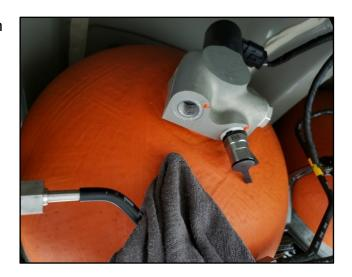
8. After removing the valve, clean the sealant from the threads in the area shown using an appropriate tool such as a pick or razor blade.
