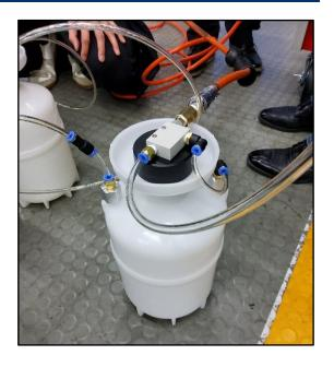
Remove any foreign material from the screw threads. Insert the suction hose only about 1cm into the thread opening. (Suction should be performed around 30 seconds.)
