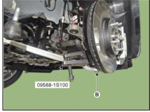
19. Remove the front drive shaft assembly (both sides).
