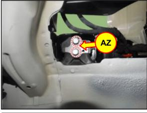
48. Lift up the vehicle to remove the traction motor and reduction gear assembly.
