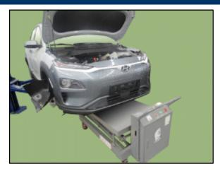
46. Remove the traction motor mounting support bracket, outlined in the figure.
