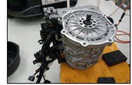
3. Stand the motor shaft upwards from the ground, then reassemble the reduction gear.
