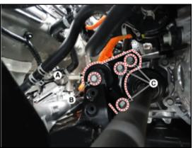
Loosen the refrigerant pipe mounting bolt 43. (AW).
