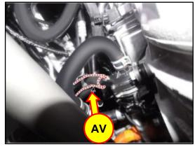
Remove the rear roll mounting bracket, 42. outlined in the figure.
