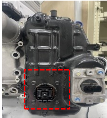
Female terminal of E-module (on DCT)
