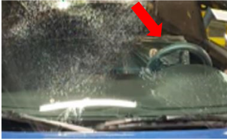
Fig. 1 Uneven Washer Nozzle Pattern on Driver Side
