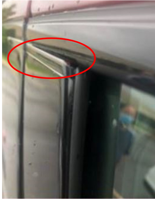
Fig. 1 Separating, Warped Or Lifting Applique
