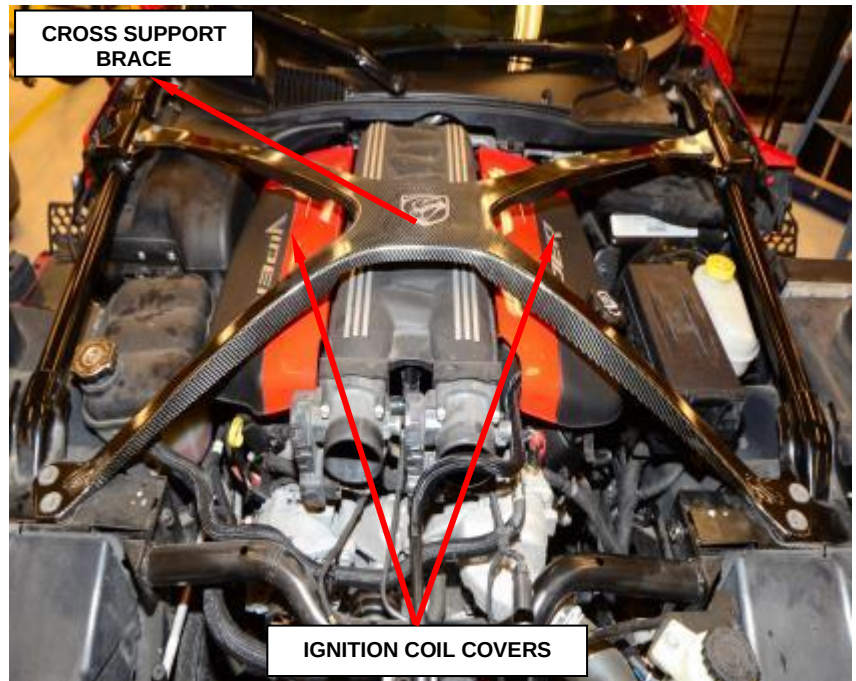
Figure 14 – Cross Support Brace
