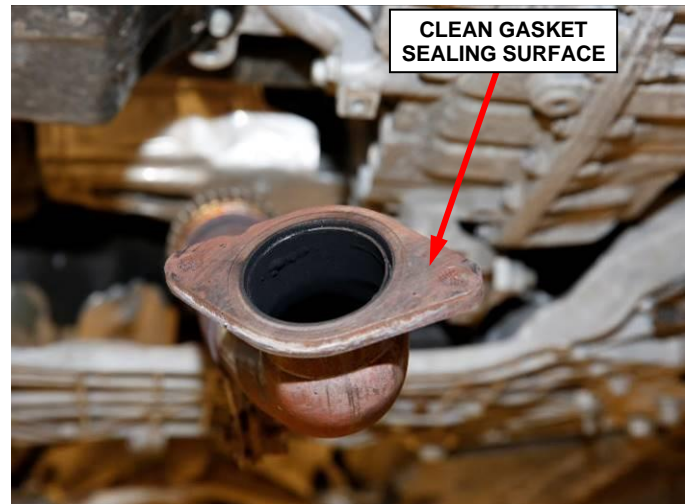
Figure 25 – Crossunder Pipe Flange
