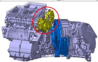
The heating and air-conditioning unit in the **G29**, left-hand drive (LHD). **Passenger Side** view
