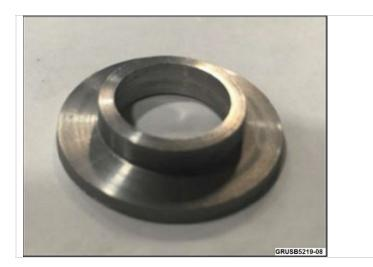
As of March 2019 production, two machined washers (shown) were added to the bottom of the inner seat rail on the driver's side (left rear) of the 60/40 split  $2^{nd}$  row seat.
