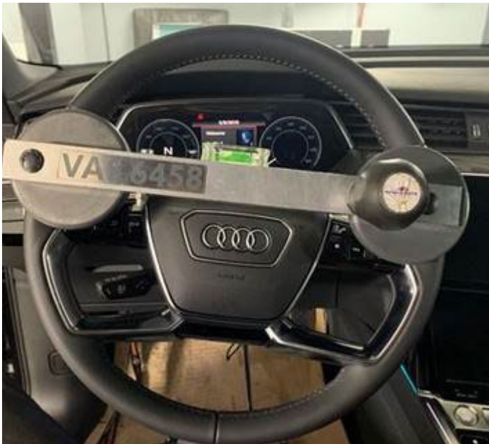
Figure 1. VAS 6458 installed with steering wheel off-center.
