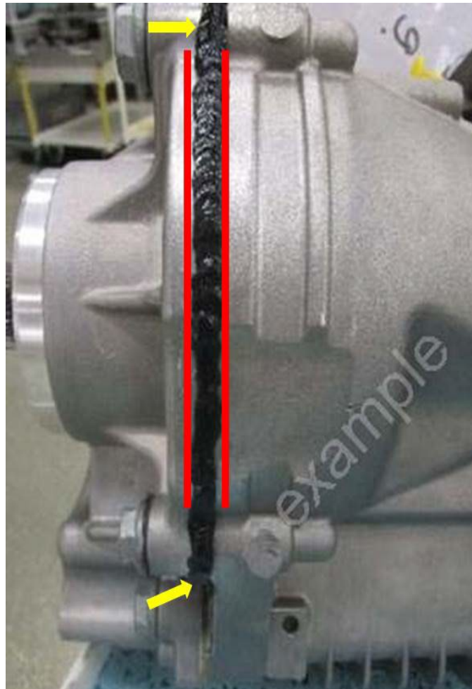
Figure 4. Silicone sealant application.
