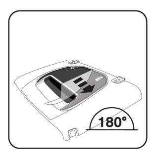
Figure 8 - Remove Premask
