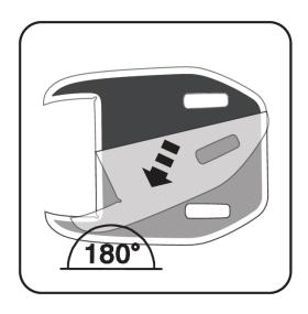
Figure 3 - Remove Paper Backing
