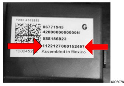
Record the serial number on the seat heater vent control module label.
